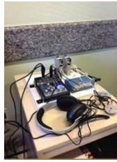
Figure 2: The portable device. We can see the grip force sensors, the amplifiers Honeywell DV10L, the data acquisition card measurement computing usb-1608GX and the headphone. The sound console is use in a other project.
