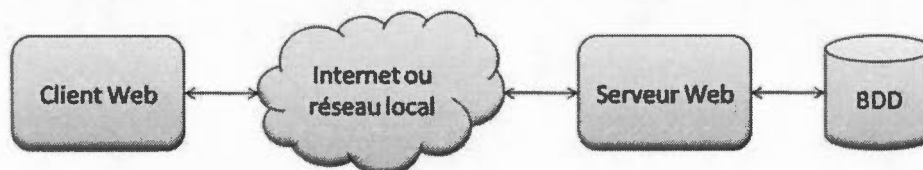
Figure V.1 : Architecture des applications Web JEE
