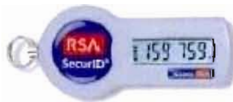
Figure 2.7: RSA SecurID® 700 hardware authenticator with One-Time Password (OTP).
