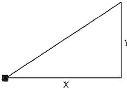
$$DD = \sqrt{\frac{X^2 + Y^2}{3}} - \left[ \frac{X^2}{3Y} \right] \ln \left[ \tan \left\{ \frac{\arctan \left( \frac{X}{Y} \right)}{2} \right\} \right]$$
