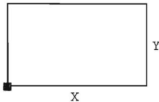
$$DD = \frac{\sqrt{X^2 + Y^2}}{3} - \left[ \frac{Y^2}{6X} \right] \ln \left[ \tan \left[ \frac{\arctan \left( \frac{Y}{X} \right)}{2} \right] \right] - \left[ \frac{X^2}{6Y} \right] \ln \left[ \tan \left[ \frac{\arctan \left( \frac{X}{Y} \right)}{2} \right] \right]$$
