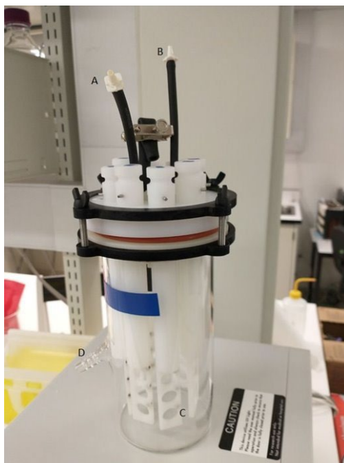
Figure 2: Bioreactor used for the incubations. The image represents one, but other two exactly like this were used for the experiments. The rock chips were installed in the spaces of each column (C). The water exits via the pipe (D) to be collected in another bottle.
