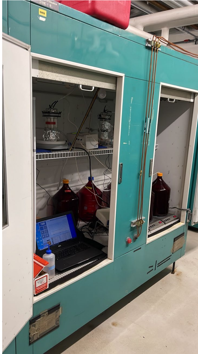
Figure S1: Closed incubation chamber used for bioreactor experiments.
