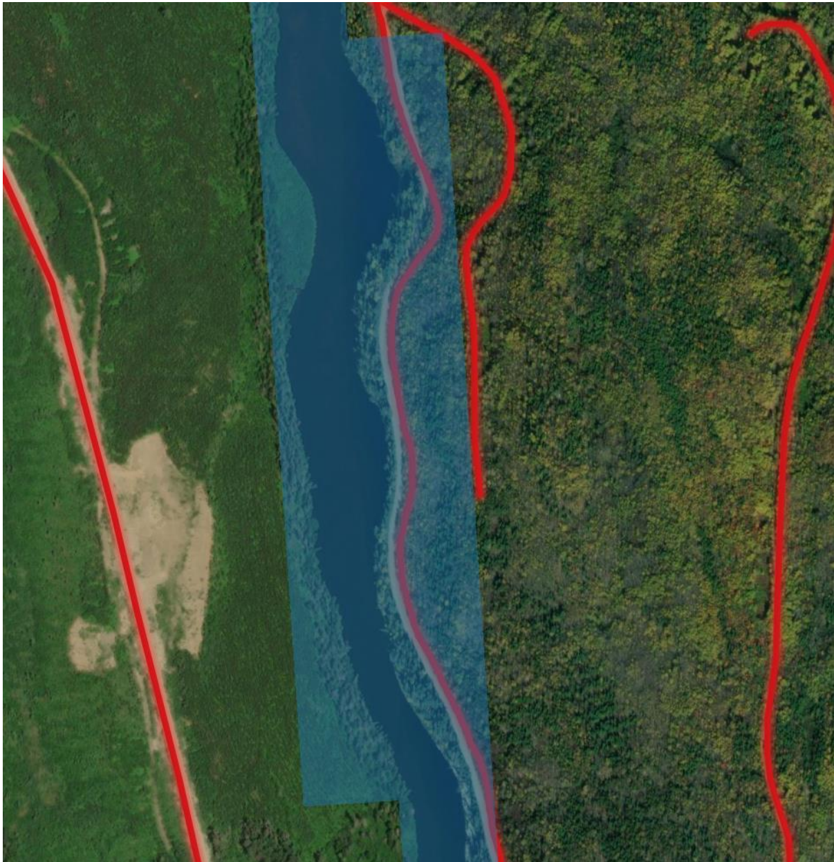
Figure B-10 : Aerial photography from Bing Maps superimposed with our initial road data (red lines) and coarse water raster (blue pixels; see section F.2.11).
