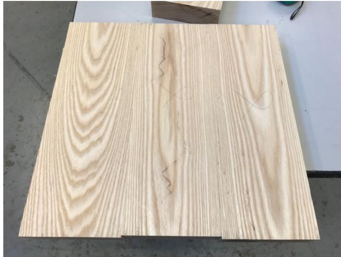
Figure 3.48 Collage assise frêne : Prototype 3
