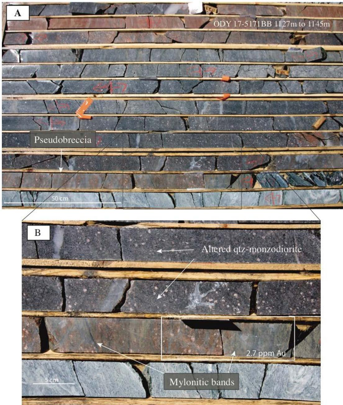
*Figure 1.8: (A) Drill core showing the hydrothermally altered quartz monzodiorite in the hanging wall of the Sladen fault, and sheared talc-chlorite-carbonate rocks in the footwall (North zone). The quartz monzodiorite developed a pseudobreccia with a matrix of greyish quartz and shows millimetric mylonitic bands within 1 m of the Sladen*
