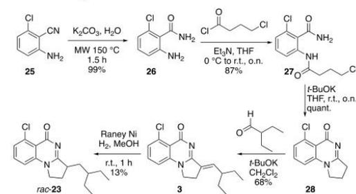
faced with the challenge of chemoselectively saturating the olefin in the presence of the aryl chloride. After testing various conditions, we found that reacting **3** with Raney nickel under a hydrogen atmosphere provided the desired saturated product **23** in low yield, albeit with the chlorine still in place.
