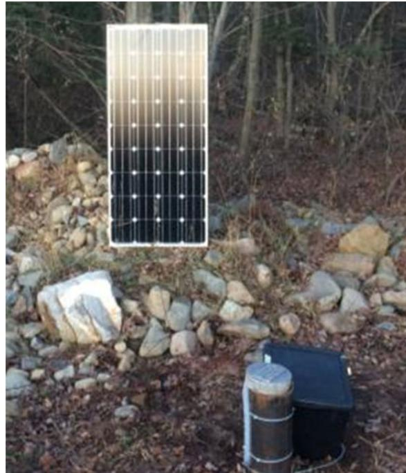
Figure 3.11 : Stand-alone low flow pumping system with solar panel.
