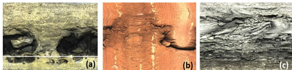
Figure 2.16 : Camera snapshots (Saint-Lawrence Lowlands) of features providing groundwater inflows: (a) dissolution conduit-dolomite; (b) discrete fracture-red shale; (c) fractured interval-dolomite
