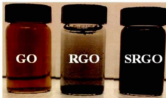
**Figure 1.** Optical images of GO, RGO and SRGO dispersed in water at the concentration of  $0.5 \text{ mg mL}^{-1}$
