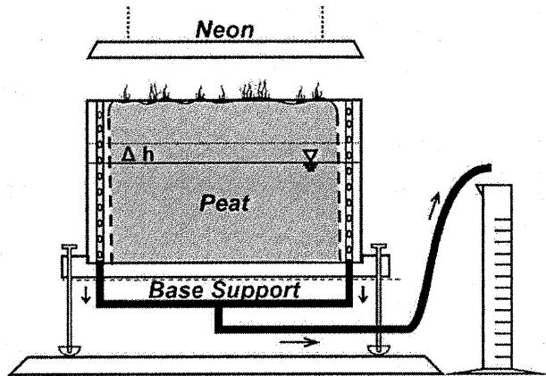
**Figure 1.4** Design of the experimental tank with an impermeable base support built for the drainage experiment to calculate specific yield variations with depth (modified from Rosa and Larocque, 2008).
