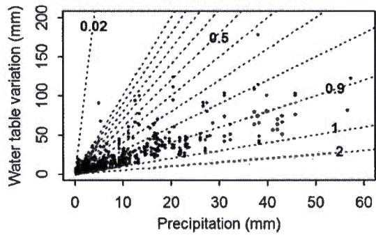
**Figure 1.7** Water table variation ( $\Delta h$ ) as a function of precipitation (P) for all sites and locations. Each point represents a single precipitation event. Dashed lines and associated value represent the ratio of  $P/\Delta h$  equivalent to  $S_y$ .
