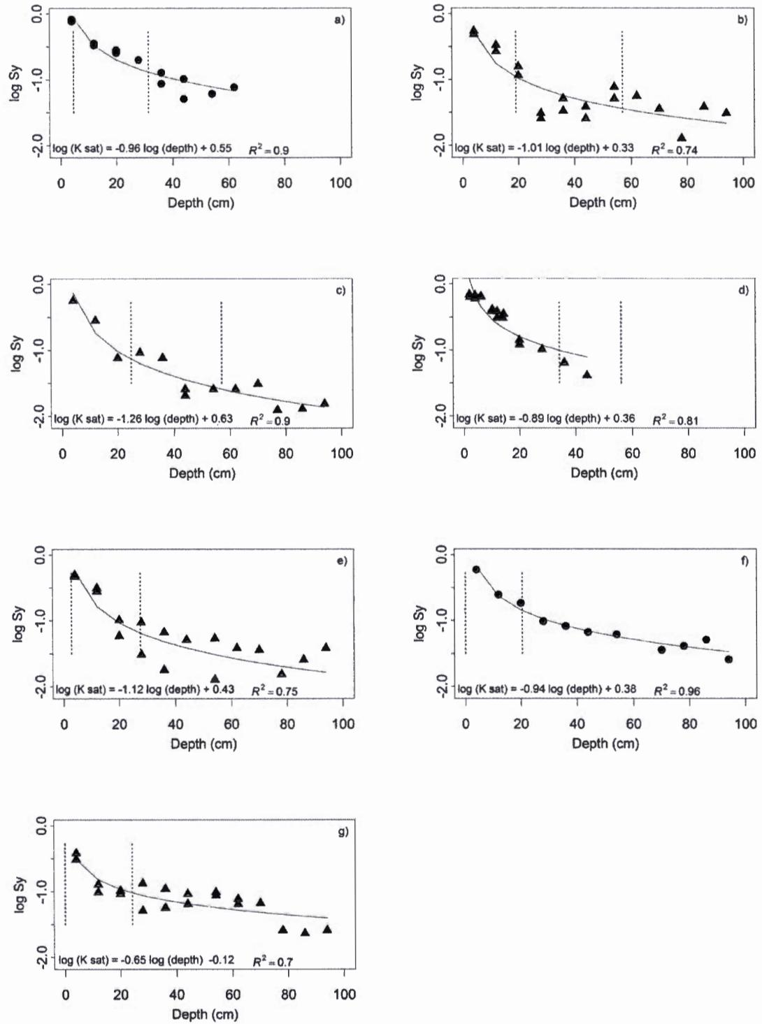
**Figure 2.9** Log-log model (black line) of  $S_y$  variations with depth in the up-gradient (black) location of the seven peatlands . The circles correspond to new data from this study, and the triangles to data from Bourgault *et al.* (2016). Black vertical dashed lines represent the maximum and minimum water table depths in the up-gradient locations.
