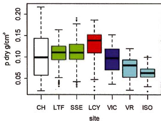
**Figure 2.4 Bulk dry density variation for all locations (up-gradient, mid-gradient, down-gradient) of the seven sites (CH, LTF, SSE, LCY, VIC, VR, and ISO). Colors show significant differences in bulk dry density between the sites. Red shows the group with the highest  $\rho_{dry}$  and light blue the group with the lowest  $\rho_{dry}$ . The group shown in white show both similarities with the green group and the dark blue group.**
