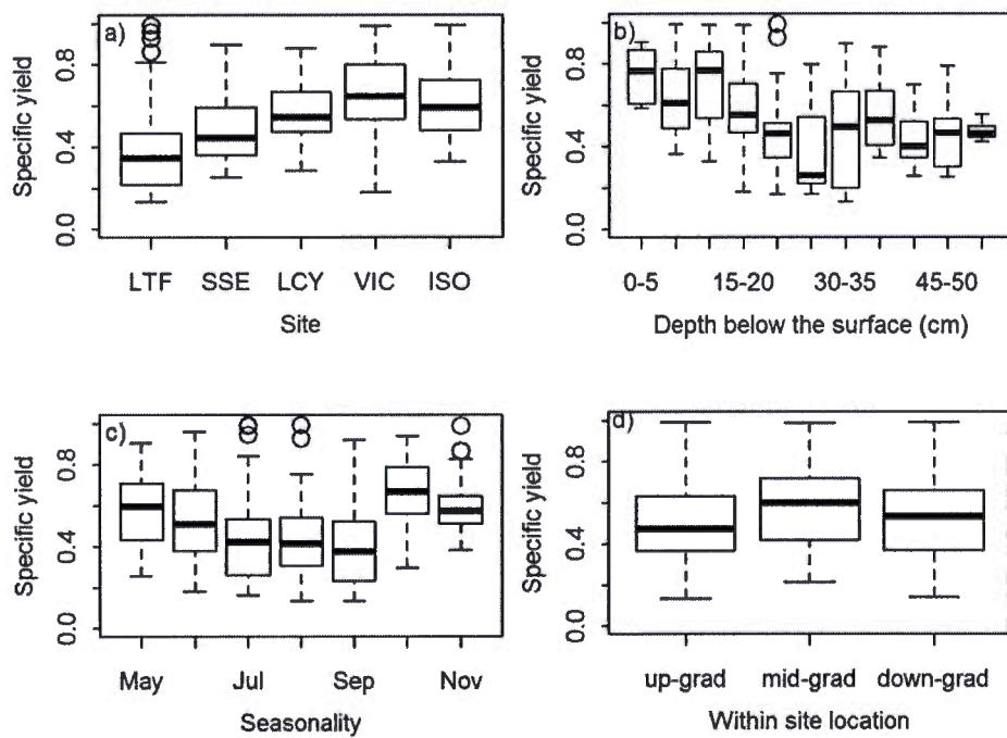
**Figure 1.9** Influence of (a) site, (b) depth below the surface, (c) seasonality (May to November), and (d) within-site location on specific yield found using the water table fluctuation method. Each box plot shows the minimum (lower bar), the first quartile (lower portion of the box), the median (bold black line), the third quartile (higher portion of the box), the maximum (upper bar), and the outliers (circles).
