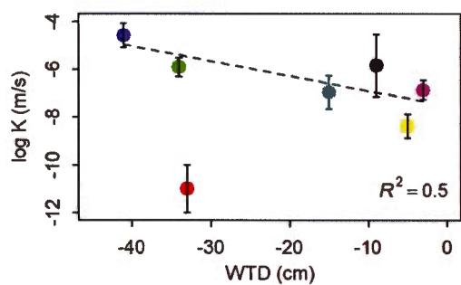
**Figure 3.7 Median (point), minimum (lower bar), and maximum (upper bar) hydraulic conductivity of the outflow zone, as a function of the median water table depth in the up-gradient piezometer (zone 1, ombrotrophic section). (Black = CH, red= LTF, green= SSE, dark blue=LCY, light blue= VIC, pink= VR, and yellow=ISO).**
