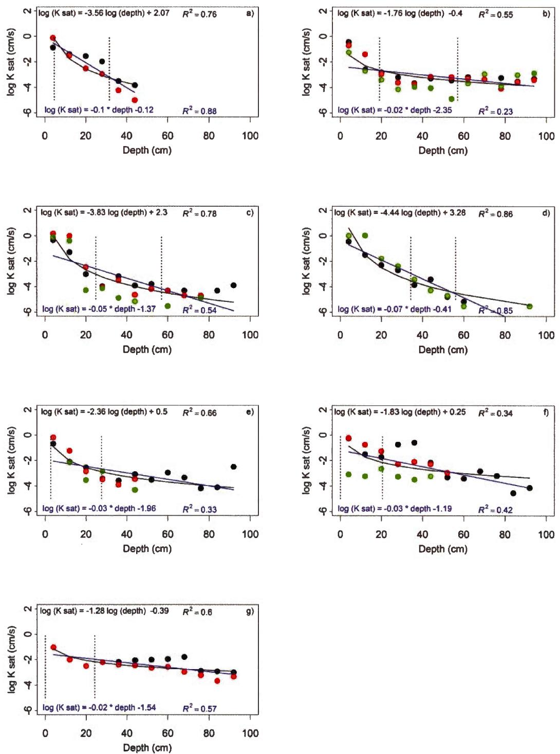
**Figure 2.7** Log K variation with depth in the up-gradient (black), mid-gradient (red) and down-gradient locations (green) of a) CH, b) LTF, c) SSE, d) LCY, e) VIC, f) VR, and g) ISO, including the log-log model (black line) and the log model (blue line), and the  $R^2$  of each. Black vertical dashed lines represent the maximum and minimum water table depths in the up-gradient locations.
