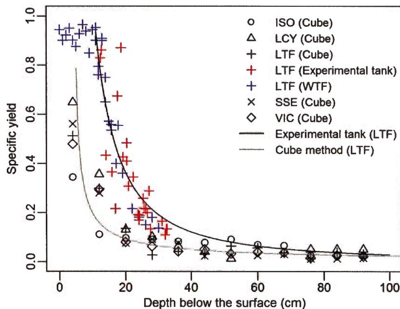
**Figure 1.6** Variation in specific yield (Sy) with depth using the small cube (mean values are plotted for each site), experimental tank (LTF only), and WTF (LTF only) methods. The black line shows the Sy–depth relationship using the experimental tank method (LTF), and the grey line shows the logarithmic Sy–depth relationship using the cube method (LTF).
