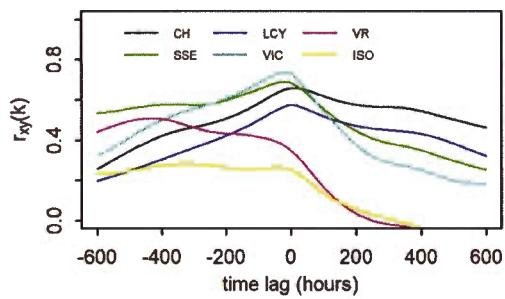
**Figure 3.11** Crosscorrelation function ( $r_{xy}(k)$ ) between the piezometer in the up-gradient portion (piezometer 1 in Figure 3.2) and the piezometer in the outflow zone (piezometer 5 in Figure 3.2).
