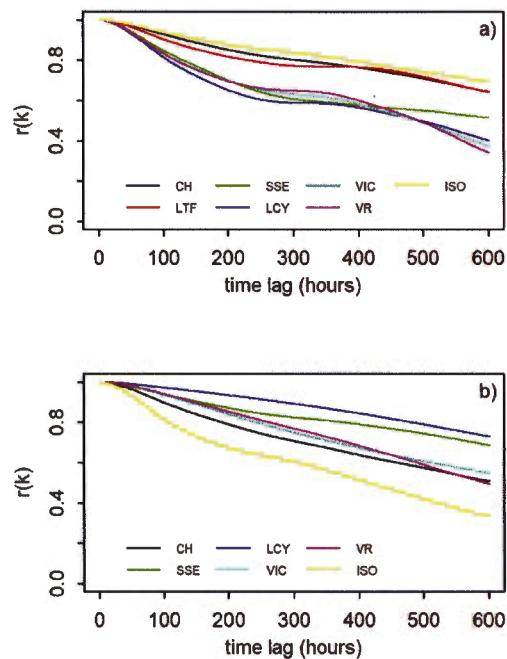
**Figure 3.10** Autocorrelation function ( $r(k)$ ) of water table depth as a function of time lag (hours) a) at the position of the ugradient piezometer (piezometer 1 in Figure 3.2) and b) in the outflow zone (piezometer 5 in Figure 3.2).
