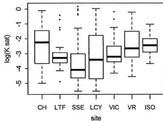
**Figure 2.6** Hydraulic conductivity variations for all locations (up-gradient, mid-gradient, down-gradient) of the sites (CH, LTF, SSE, LCY, VIC, VR, and ISO).
