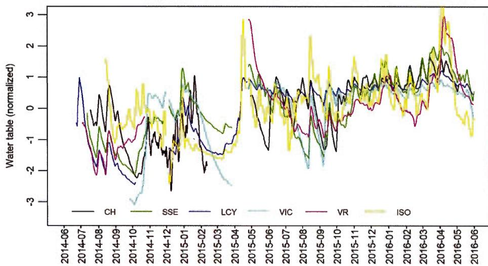
**Figure 3.6 Normalized (standard score) water table depth in the outflow zones (piezometer 6 on Figure 3.2) of the aquifer for sites CH, SSE, LCY, VIC, VR, and ISO, from June 2014 to June 2016.**
