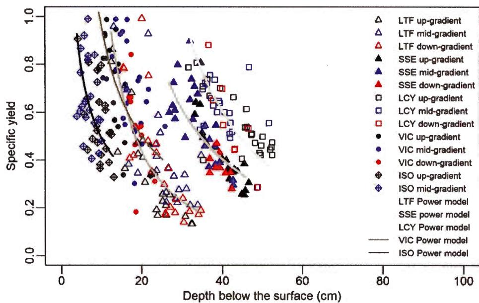
**Figure 1.8 Variation in specific yield estimated using the power law model applied to the WTF method as a function of depth below the surface for all peatlands and all locations (up-gradient, mid-gradient, and down-gradient)**
