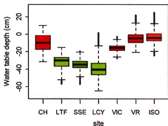
**Figure 2.2 Water table depths (WTD) for all locations (up-gradient, mid-gradient, down-gradient) of the seven sites (CH, LTF, SSE, LCY, VIC, VR, and ISO) from June 2014 to May 2016. Colors show significant differences in WTD between the sites. Red boxplots show the significant different group composed of CH, VIC, VR, and ISO whereas green boxplots show the second group composed of LTF, SSE, and LCY.**
