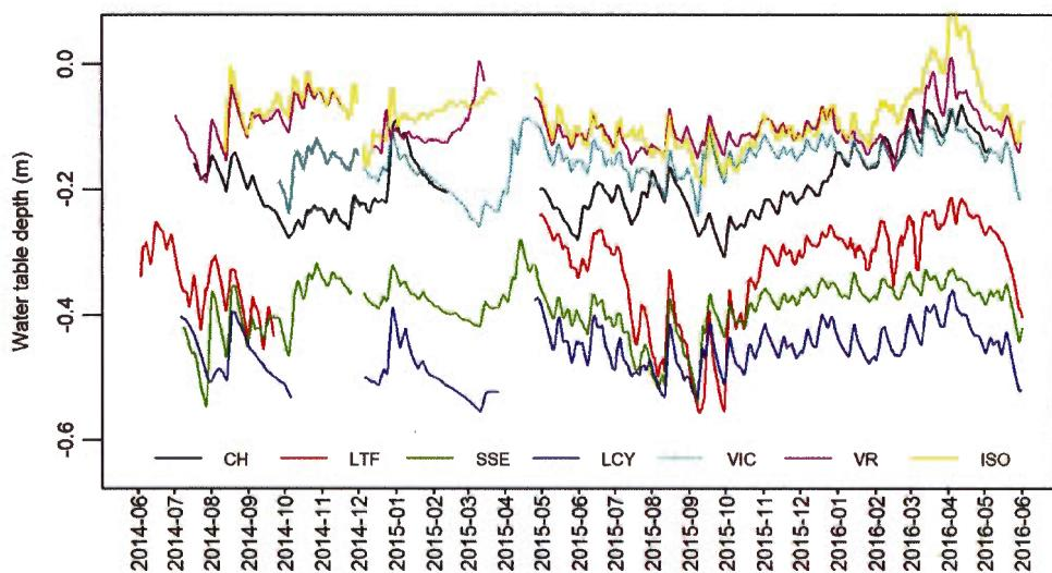
**Figure 3.3 Temporal evolution of the water table depth in the up-gradient piezometer (piezometer 1 in Figure 3.2) of each studied peatland, from June 2014 to June 2016.**
