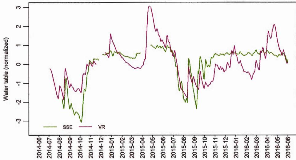
**Figure 3.5** Normalized (standard score) water table depth in the inflow zones (piezometer 5 in Figure 3.2) of the aquifer for sites SSE and VR, from June 2014 to June 2016.
