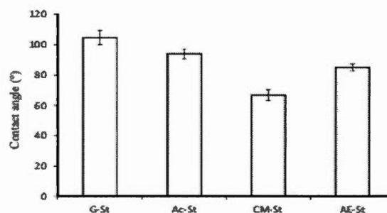
Fig. 3. Water contact angle measurement for insert coating films of Gelatinized starch (G-St), Acetate starch (Ac-St), Carboxymethyl starch (CM-St) and Amino-Ethyl starch (AE-St) ( $n = 3$ ).
