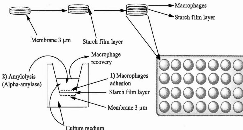
Scheme 1: Design of device and procedure with adhesion (1) and amyolysis (2) steps for fast recovery of macrophages.
