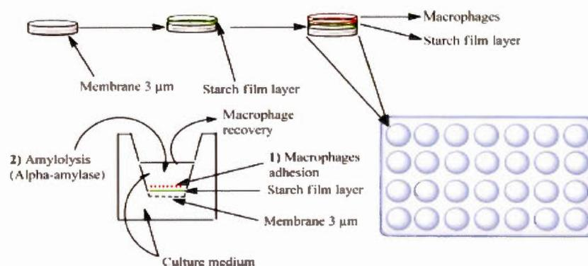
**Scheme 1.** Design of device and procedure with adhesion (1) and amylolysis (2) steps for fast recovery of macrophages.
