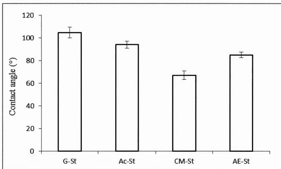
Fig 3: Water contact angle measurement for insert coating films of Gelatinized starch (G-St), Acetate starch (Ac-St), Carboxymethyl starch (CM-St) and Amino-Ethyl starch (AE-St) ( $n = 3$ ).
