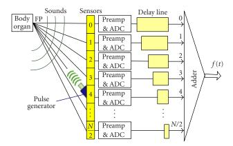
FIGURE 3: Simplified schematic of the pipelined digital beamforming.
