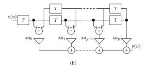
FIGURE 9: Realization of FIR filter: (a) simple direct structure and (b) direct structure for a linear phase filter.
