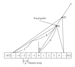
FIGURE 4: Dynamic focusing and steering delay.
