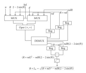
FIGURE 7: Block diagram of the delay time distance calculation.
