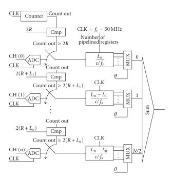
FIGURE 6: Block diagram of the pipelined sampled-delay.
