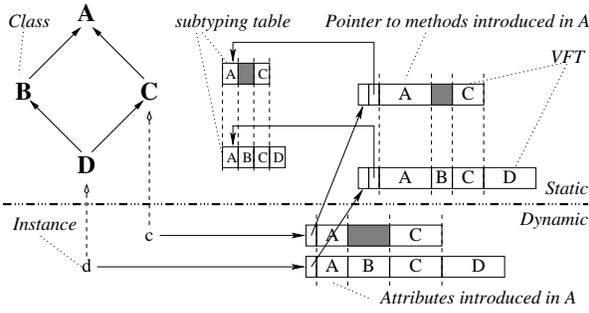
**Figure 1: Implementation of Classes and Instances with Coloring**
