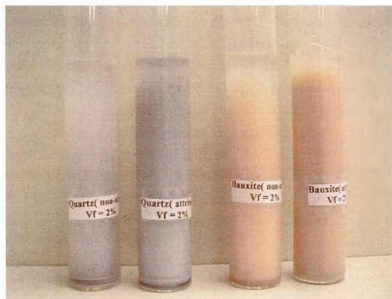
Figure 1.1 Comparing the attrited and non-attrited mineral slurries, from left to right: a) non-attrited quartz. b) attrited quartz. c) non-attrited bauxite d) attrited bauxite.
