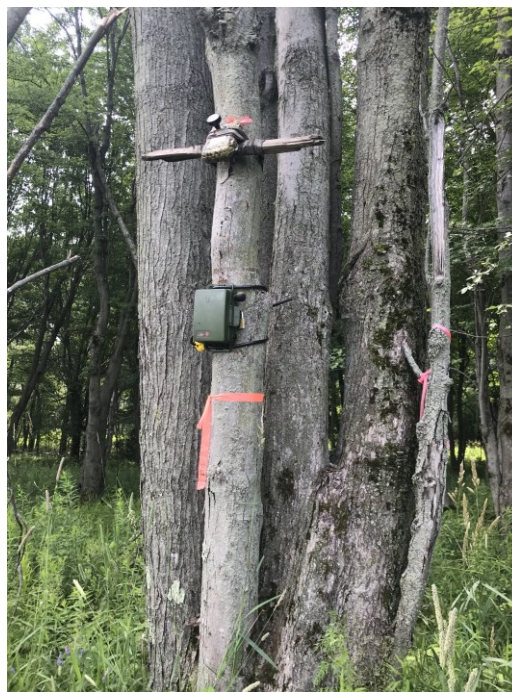
Figure 2.2 Picture of a recording station at the forest’s edge. The Anabat® was installed at a 45° angle pointing upward, and at a 2-meter height from its microphone to the ground. The SM4® was positioned below the Anabat®, at 50 cm between the microphones of each recording device (Grinfeder et al. , 2022; Charbonneau et al. , 2023).
