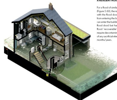
Figure 5.61: A resilient house (during/after)
