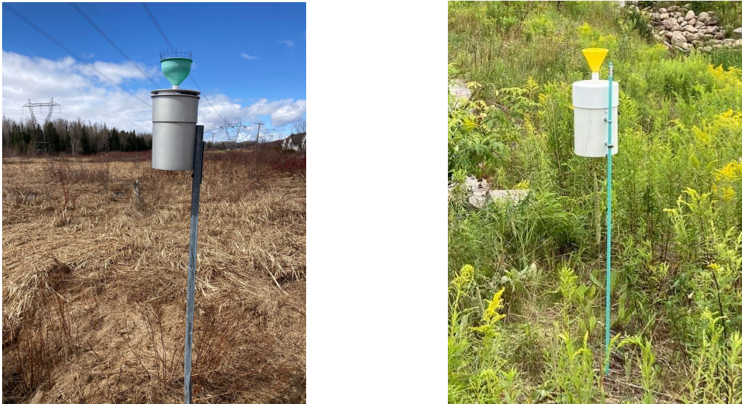
Figure 80 : On the left, Palmex® collector used at the lake Saint-Charles station. On the right, homemade rainfall collector installed in the catchment.
