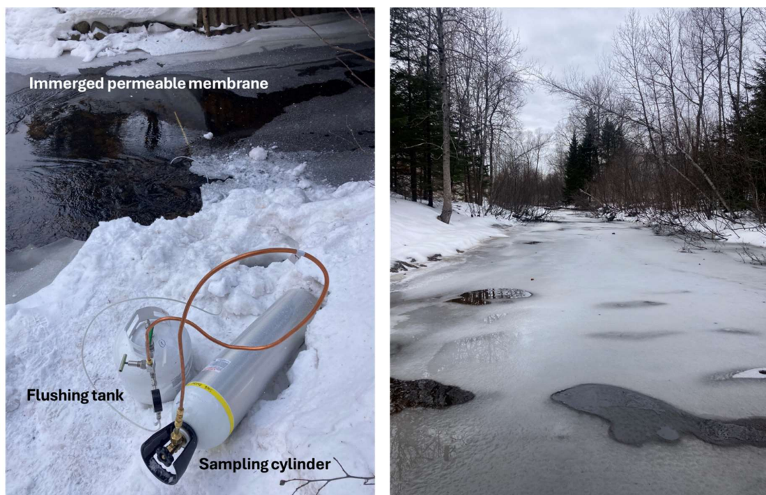
Figure 56: Apparatus used for in-situ sampling of ^{85}\text{Kr} (left) and river aspect during fieldwork showing the partial ice cover close to SW4 (right).
