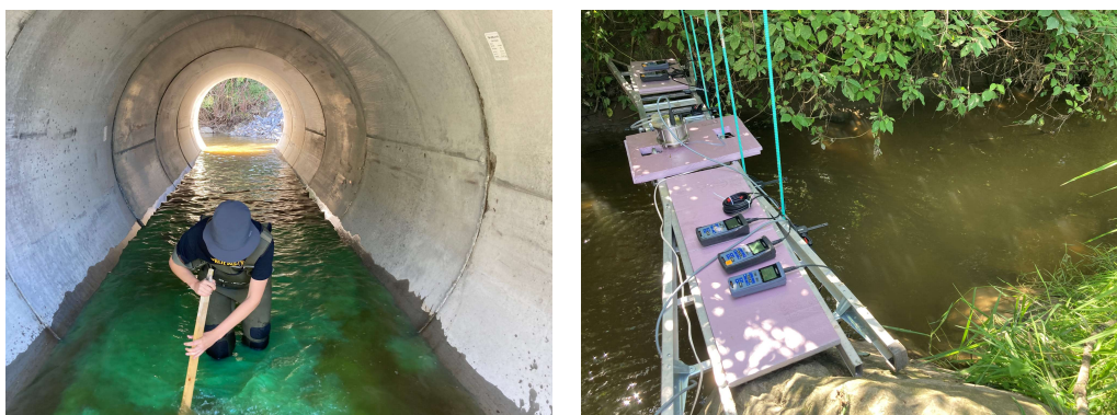
Figure 18: On the left : picture of the stream at the injection site (under a small culvert). We ensured tracer homogeneity by manually fanning the water under the culvert. On the right : picture of the restitution site with the equipment used to monitor solute concentration.
