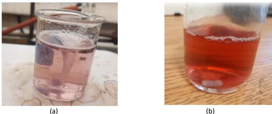
Figure 13. The color changes after adding the first reducing agent (a), and again after 90 minutes at 80 degrees (b).
