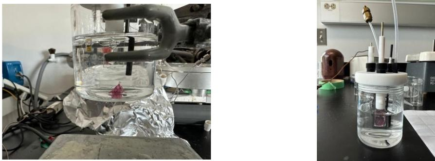
Figure 4.1. Left: The film has detached and fallen into the electrolyte, demonstrating its instability. Right: The film remains intact and adhered to the surface after being stabilized with a surrounding application of Transparent nail polish is a film formed from a nitrocellulose-based polymer in solution.
