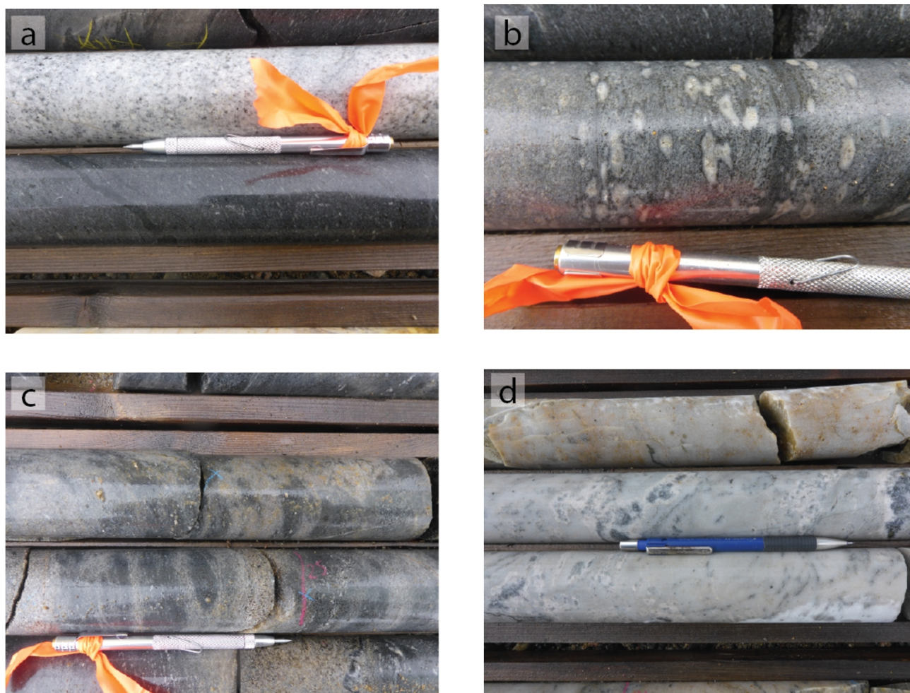
Figure 7: Core from drillhole HEN-228, Izok Lake deposit: a) white leucogranite and dacitic tuff; b) porphyroblasts with a white mica core and white feldspar and chlorite rims; c) pseudoclastic/patchy chlorite texture in a sericite-altered rhyolite; d) sericite-altered, leached rhyolite.
