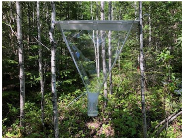
Figure 1.4 IBL flight intercept trap used to sample saproxylic beetles in hardwood and mixedwood stands of our study.
