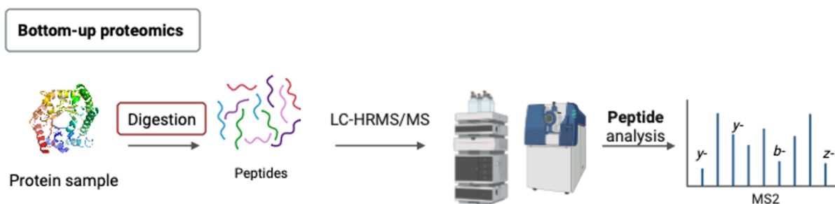
Figure 1.10 Simplified bottom-up proteomics workflow
