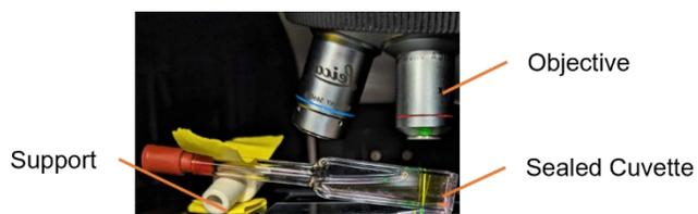
Figure 3.11. Experimental set-up to acquire resonance Raman spectrum in solution.
