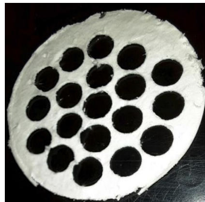
Figure 4.7 (A) Distribution of impregnated MAMA on 37 mm GFF; (B) Distribution of collected airborne MDI on impregnated MAMA GFF; (C) Sampling pattern. Percentages (A and B) describe the MAMA or MDI distribution (normalized vs the highest value (100%) of mass per circular subsection)
