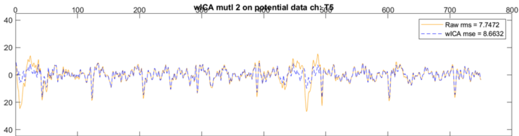
Figure 2.2: wICA artifact removal algorithm. One-channel raw EEG data (in yellow) and the denoised signal using wICA (in blue). The root-mean-square of each signal is also stated on the top-right corner.
