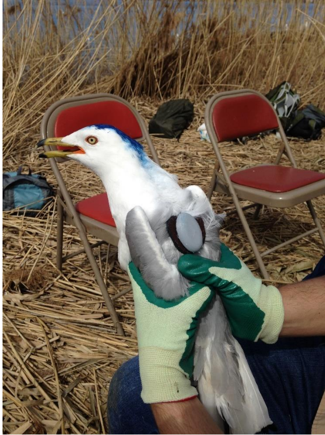
Figure C.1 Ring-billed gull carrying a passive air sampler (PAS) attached using a customized harness in the middle of its back.
