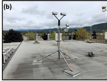
Figure 2.3: Instrumentation setup at the downtown Terrace station (UNBC campus rooftop), namely (a) a MRR2, (b) a OTT Parsivel 2 and a Goodrich 0872F1 ice detector, and (c) the complete weather station with the setup datalogger and a HOBO tipping bucket precipitation gauge.
