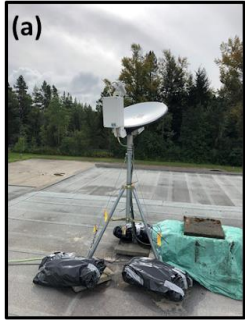
Figure 2.3: Instrumentation setup at the downtown Terrace station (UNBC campus rooftop), namely (a) a MRR2, (b) a OTT Parsivel 2 and a Goodrich 0872F1 ice detector, and (c) the complete weather station with the setup datalogger and a HOBO tipping bucket precipitation gauge.
