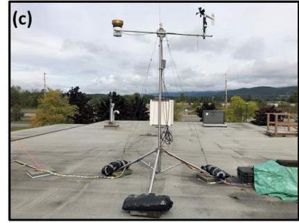
Figure 2.3: Instrumentation setup at the downtown Terrace station (UNBC campus rooftop), namely (a) a MRR2, (b) a OTT Parsivel 2 and a Goodrich 0872F1 ice detector, and (c) the complete weather station with the setup datalogger and a HOBO tipping bucket precipitation gauge.
