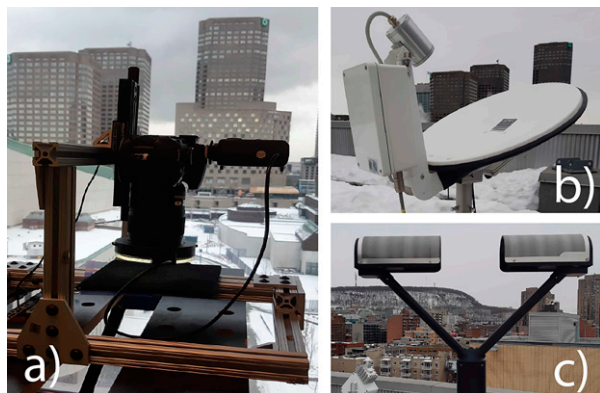
FIG. 5. (a) Camera setup used at PK-UQAM station for photography, (b) MRR-2, and (c) OTT Parsivel 2 laser-optical disdrometer located at PK-UQAM station.
