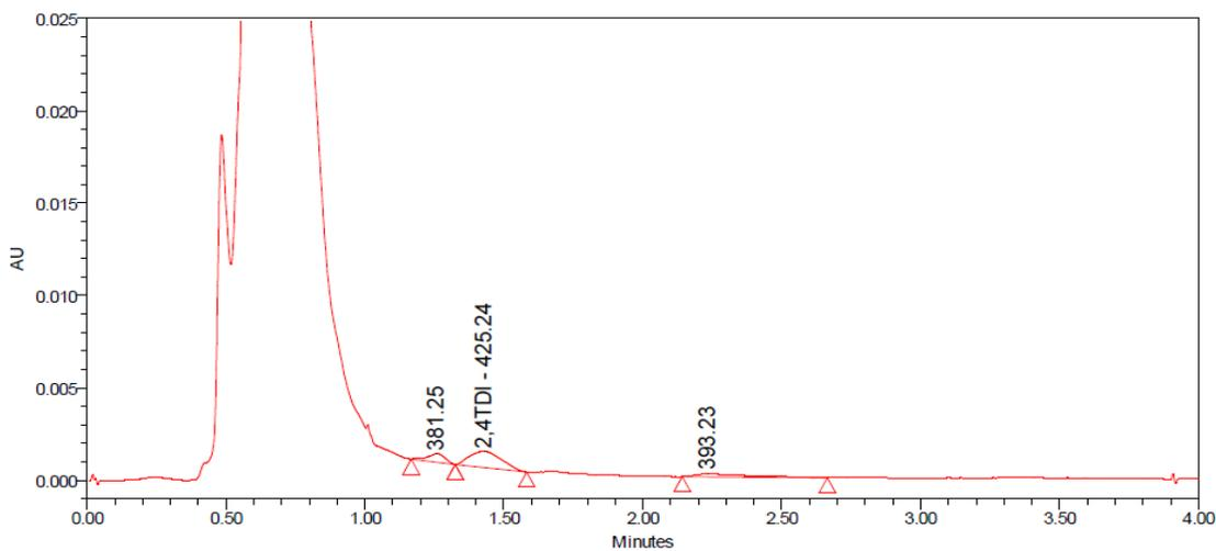
b) filter wetted with synthetic sweat solution after 12 hrs contact with the foam sample
