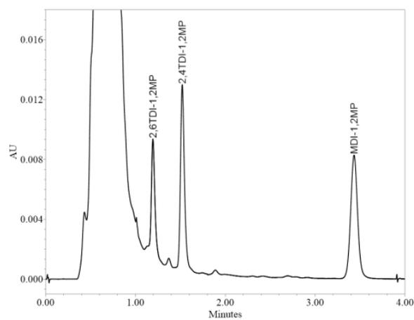
b) MS standard chromatogram with Extract Ion Chromatograms (XIC) for 2,6-TDI-1,2-MP (at 1.186 min), 2,4-TDI-1,2-MP (at 1.506 min) and MDI-1,2-MP (at 3.392 min)
