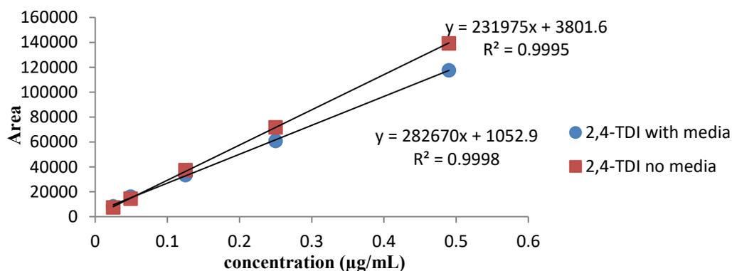
**Figure 3.3** Calibration curve for the 2,4-TDI-1,2MP standards prepared by spiking the wetted impregnated filter (with media) or into a 1,2-MP solution (no media).
