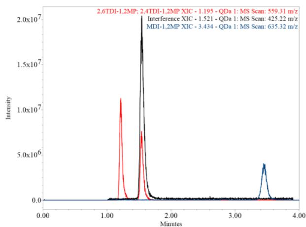
Figure 2.2 UV (a) and MS (b) chromatograms of 2,6-TDI-1,2-MP, 2,4-TDI-1,2-MP, MDI-1,2-MP
