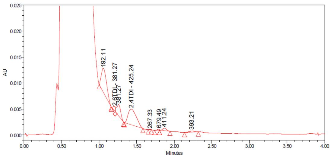
a) filter blank wetted with synthetic sweat solution after 12 hrs exposed to ambient air.
