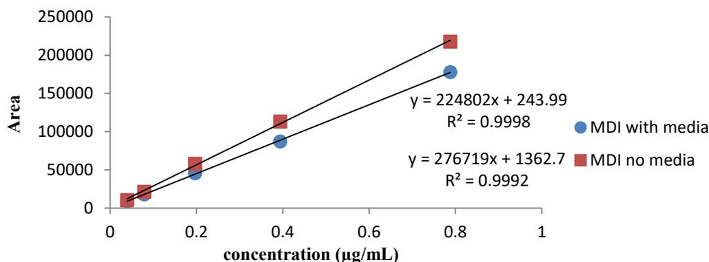
**Figure 3.4** Calibration curve for the MDI-1,2MP standards prepared by spiking the wetted impregnated filter (with media) or into a 1,2-MP solution (no media).
