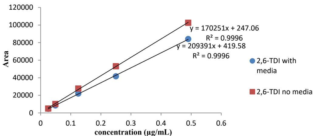
**Figure 3.2** Calibration curve for the 2,6-TDI-1,2MP standards prepared by spiking the wetted impregnated filter (with media) or into a 1,2-MP solution (no media).
