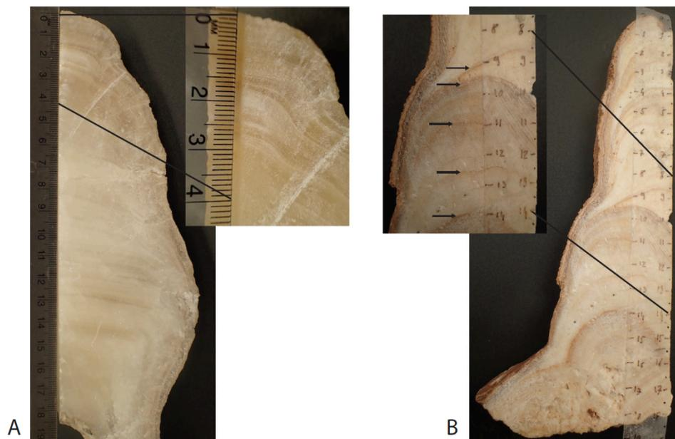
Figure B.5 Photographs of sections in stalagmites showing (a) growth bands with a yearly resolution (sample from Vancouver Island, Canada; cf. Marshall *et al.* 2009) and (b) interannual water supply variation in relation with drought cycle (Algarve basin, Portugal; cf. Ponte *et al.* 2017). Scale in centimeters.
