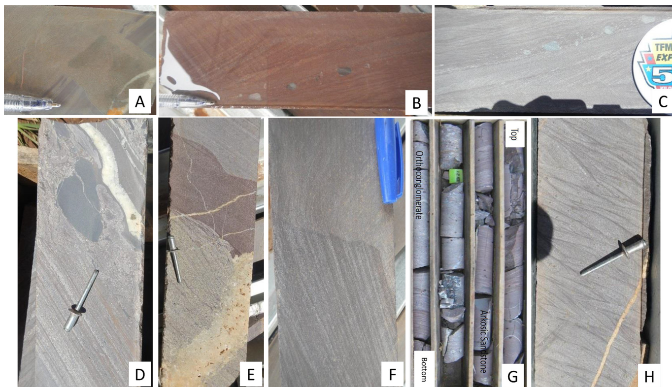
Fig. 4. Sedimentary structures and soft sediment deformation structures: (A) Neptunian dykes per descensum and sills by injection shales; (B) and (C) Scour and toll mark, (D) Balls and pillows structure, (E) Load structure, (F) Erosional surface, (G) Bouma sequence; (H) Cross bedding in arkosic sandstone.
