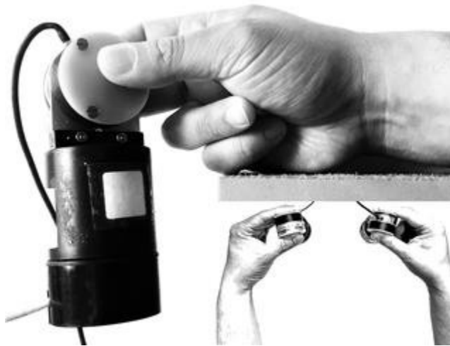
Fig 2.1. Grip force sensor held by means of a tri-digital pinch. Arm support extends to the fifth metacarpal head while the sensor remains hanging in the gap. The sketch in detail shows the symmetrical bimanual positioning and displays the neutral position of flexion/extension of the wrists.
