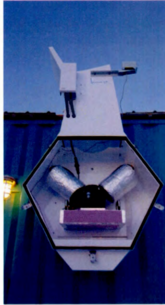
FIGURE 1.4: FIRR installation at OPAL
