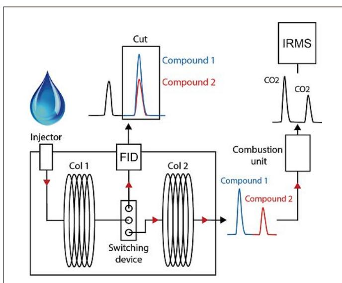
2D-GC-IRMS configuration for carbon isotope analysis. The switching device after the first column directs by default the flow to the FID detector. Compounds of interest are sent to the second column by heart-cuts defined according to their retention time on the first column, and then to the IRMS detector.
