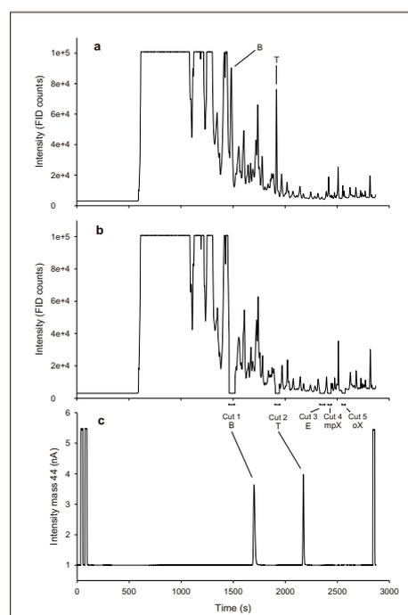
2D-GC-IRMS analysis of a gas-phase sample. a) FID chromatogram without heart-cuts, b) FID chromatogram with heart-cuts for BTEX and c), the corresponding IRMS chromatogram. Only benzene (B) and toluene (T) were sent to the IRMS. Reprinted with permission from Elsevier, Ponsin *et al.*, *J. Chromatogr. A* **2017**, *1492*, 117.
