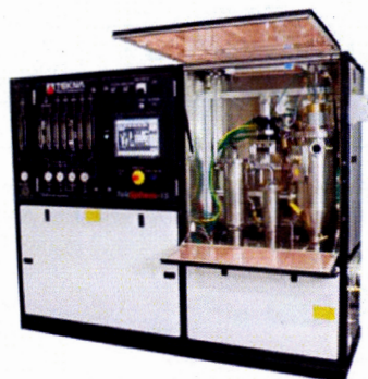
Figure 4.11 Laboratory induction plasma torch system, 15 kW (Tekna, TekNano-15).
