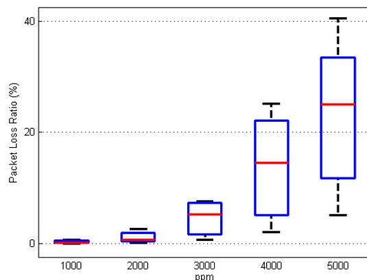
FIGURE 14. Packet loss ratio statistics of CLRPL at different traffic loads.
