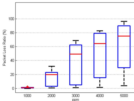
FIGURE 13. Packet loss ratio statistics of RPL at different traffic loads.
