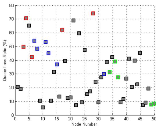
FIGURE 12. Nodes Queue loss ratio in the topology made by RPL.
