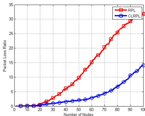
FIGURE 15. Packet loss ratio at different network sizes.
