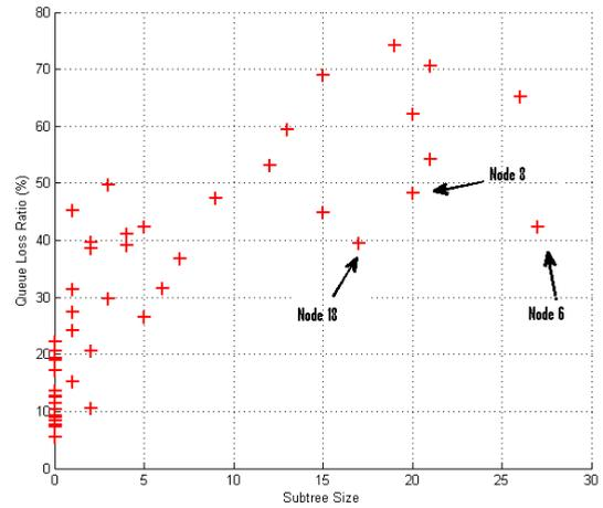
FIGURE 9. Subtree size to Queue loss ratio in RPL.
