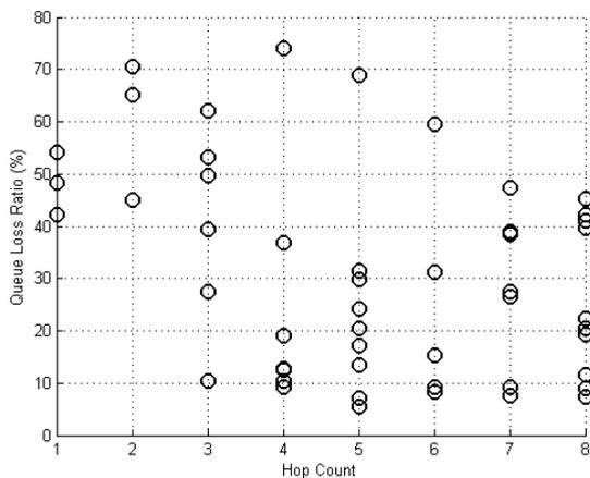
FIGURE 11. Distance from border router to Queue loss ratio in RPL.
