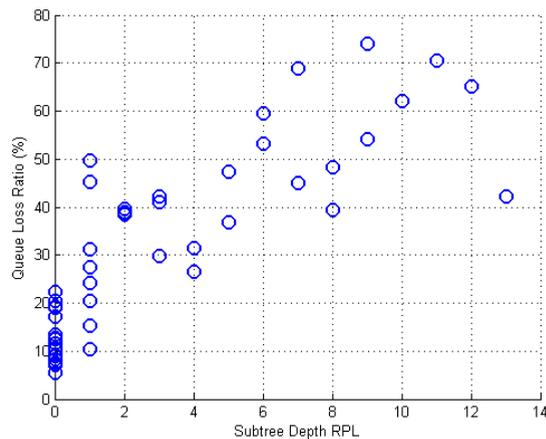
FIGURE 10. Subtree depth in RPL to Queue loss ratio.
